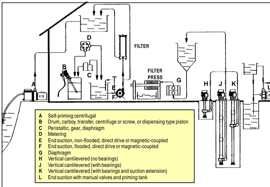
Reference E in the above illustration indicates that the horizontal pump would have to be manually primed at least the first time used, and a foot valve (check valve) should be used on the suction side of the pump to maintain the primed condition when the pump is not operating
