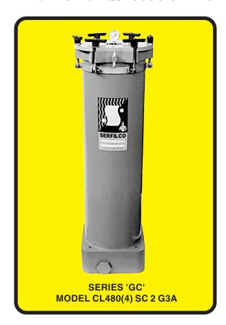
Series 'GC' chambers feature a precision CNC machined base and molded cover. The innovative base design has 2" inlet and outlet ports providing low pressure differential. The base includes 3/4" plugged drain ports for ease of maintenance. The shell is cemented to the machined base to eliminate leakage and warping. The cover includes a vent valve, 0-60 psi pressure gauge with guard assembly, and an FRP cover plate. The cover is secured with swing
